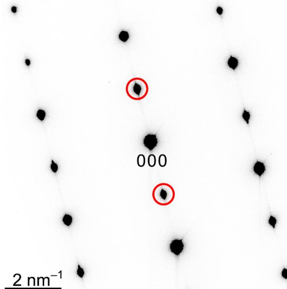
The intensity of these spots is similar to many of the other diffracted beams. This confirms how dynamical scattering can make it difficult to interpret the intensities of diffracted beams in a zone axis diffraction pattern.
