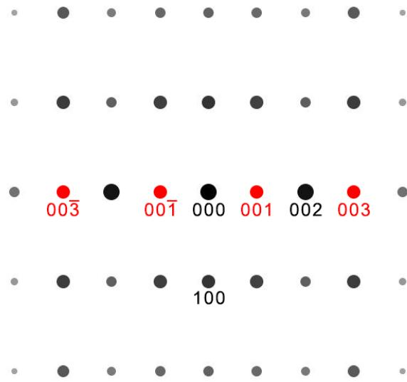
iii) The double diffraction created spots closest to the direct beam correspond to  $\mathbf{g}$  vectors of either:
